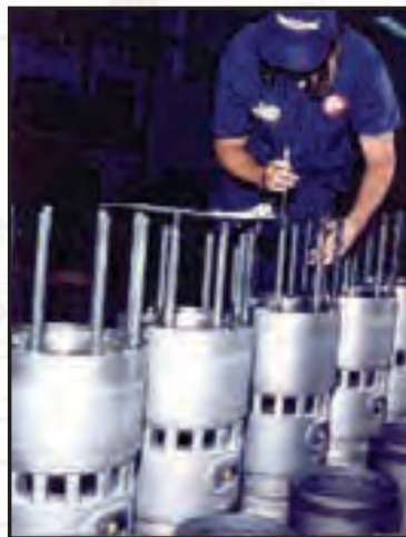
Precision Inspection of all Liners
